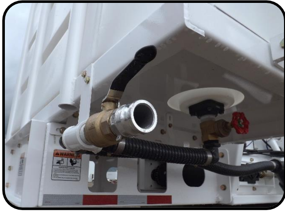
Figure 5. Water tank bottom load cam lock fitting.
