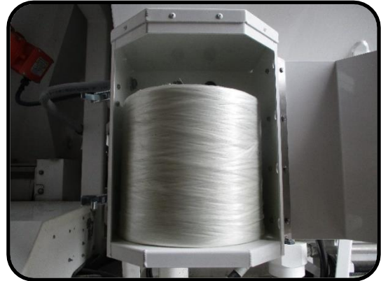
Figure 18A & 19B. Fibre feeder.
