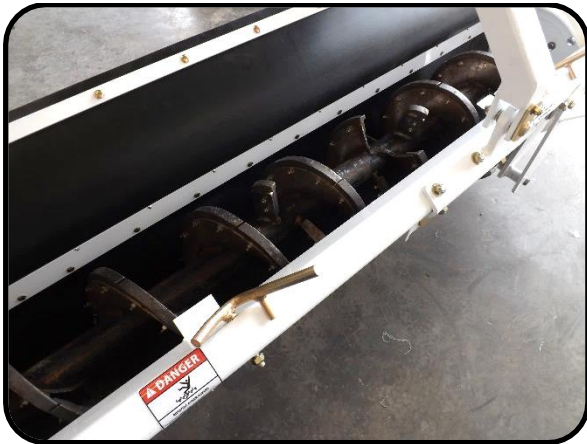
Figure 9. Auger cover open for cleaning.
