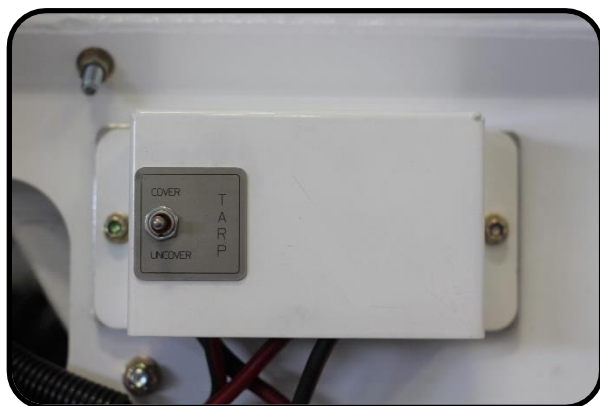
Figure 26. Tarp control switch.
