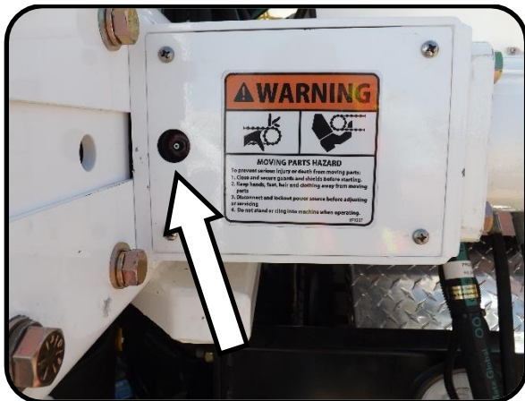
Maintenance 7. Rear conveyor shaft grease, right.
