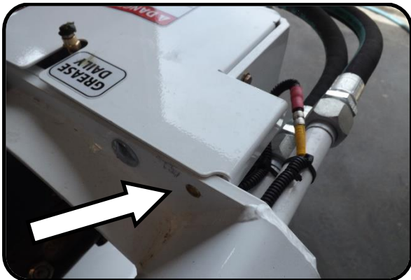
Figure 10. Auger cover safety switch.
