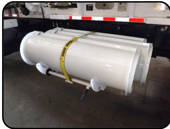
Figure 27. Extension chute carrier and chutes.
