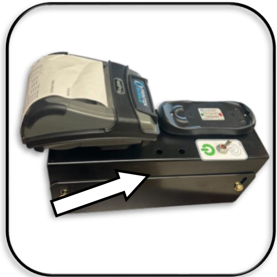
Figure 20. Remote receiver / printer stand master electrical switch
