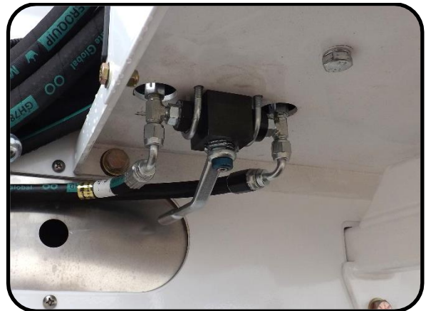
Valve Location 9. Free swing selector valve.
