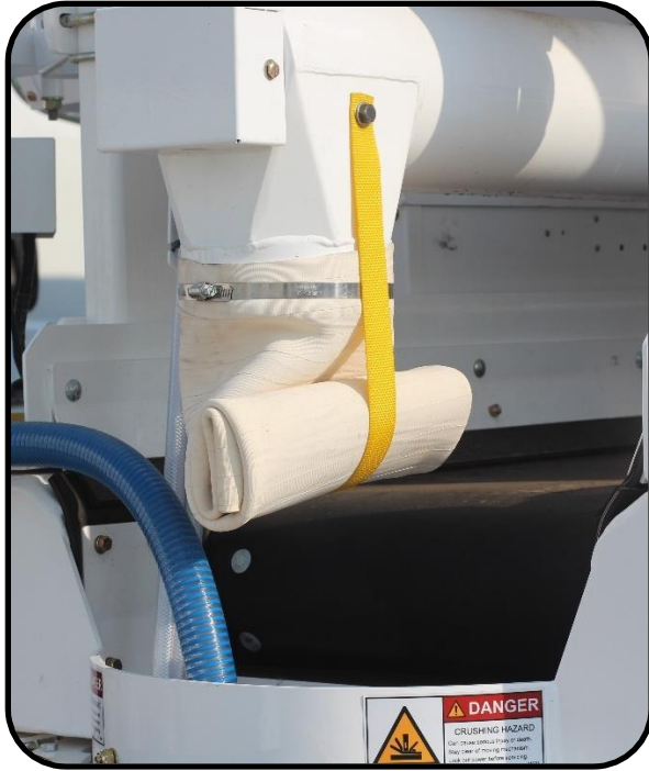
Figure 21. Cement drop tube.
