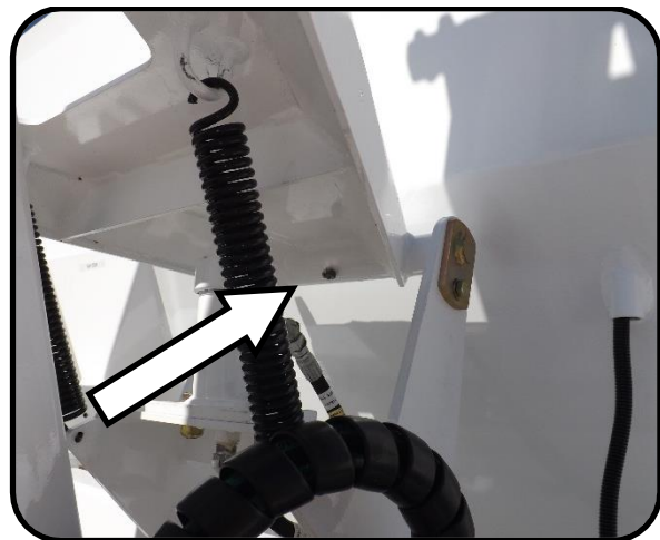
Maintenance 10. Lock arm grease.
