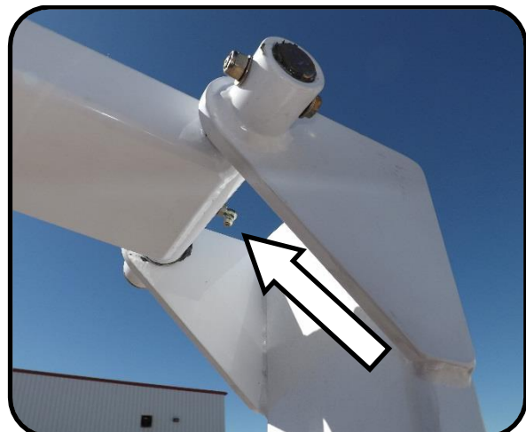
Maintenance 11. Upper lift link grease.
