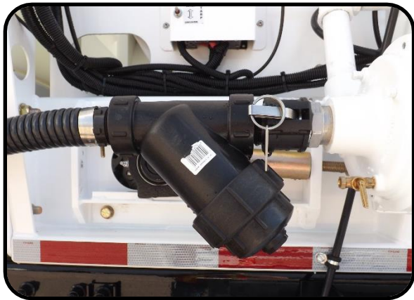
Maintenance 17. Clean water Y strainer.
