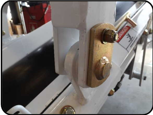
Figure 13. Lower link auger pivot.
