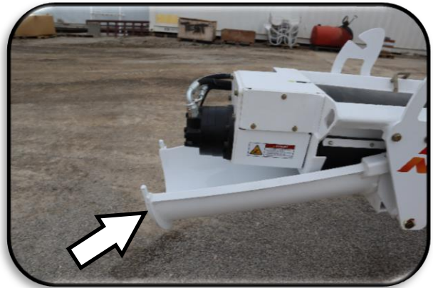
Figure 15. Mix auger transition chute.
