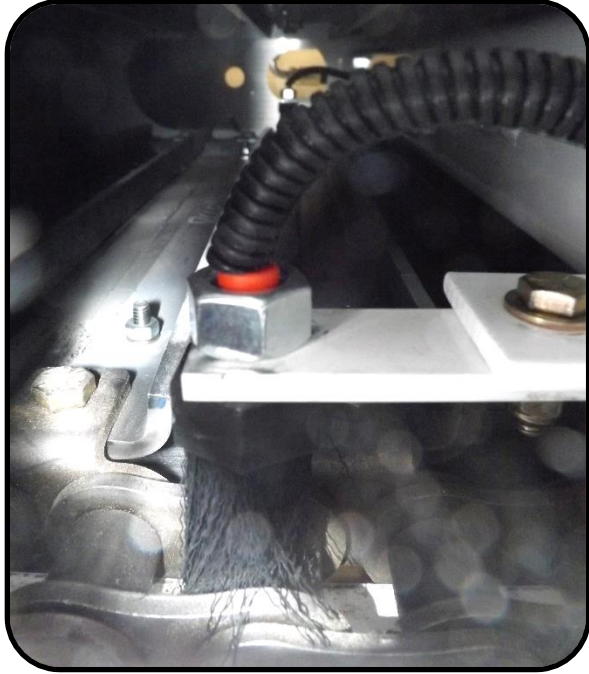
Maintenance 16. Conveyor chain brush check.
