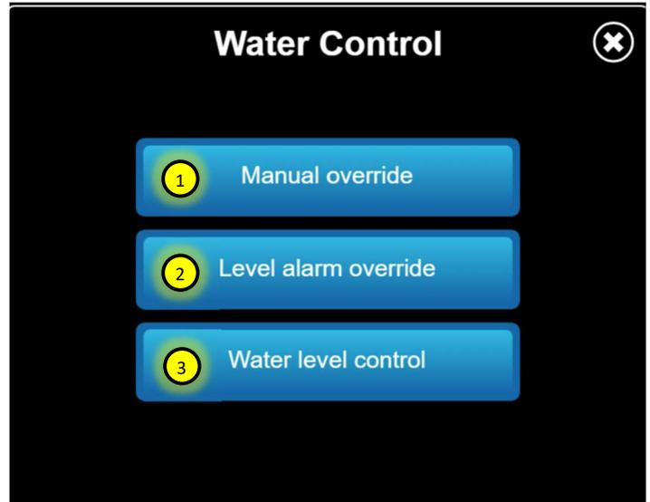
4. Calibrate the low water level setting. This can be done with a small amount of water in the tank or empty. It depends on where the user wants the 0% reading to start.
