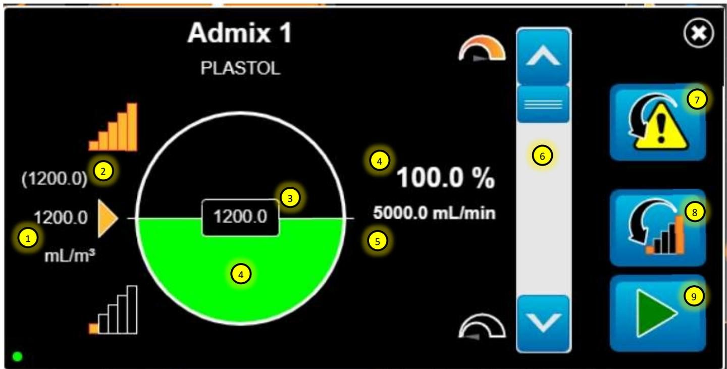
1. Admix production rate currently set by the operator. If the arrow is orange, then the production rate selected is different from the mix design.
