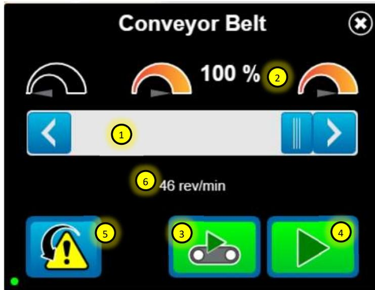
1. Speed control slider. Right arrow to increase speed, left arrow to decrease speed.
