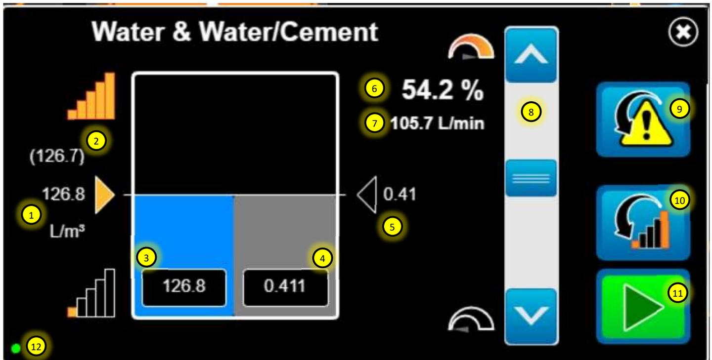
1. Water production rate currently set by the operator. If the arrow is orange, then the production rate selected is different from the mix design.
