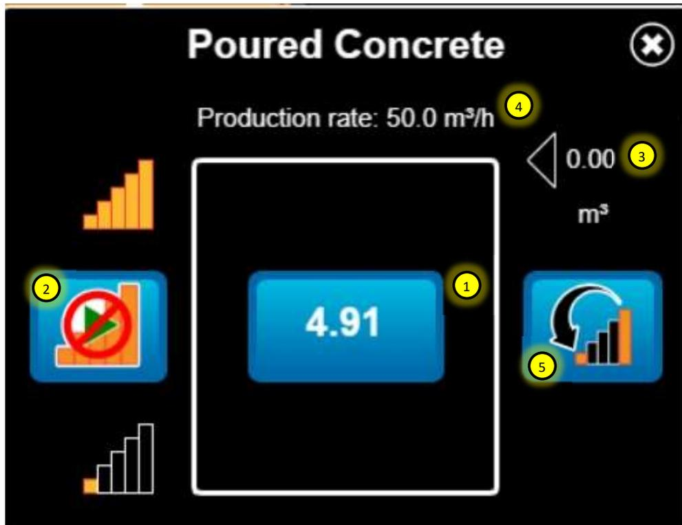
1. Current volume of concrete produced. This can be pressed to show table of current totals of each mix ingredient.
