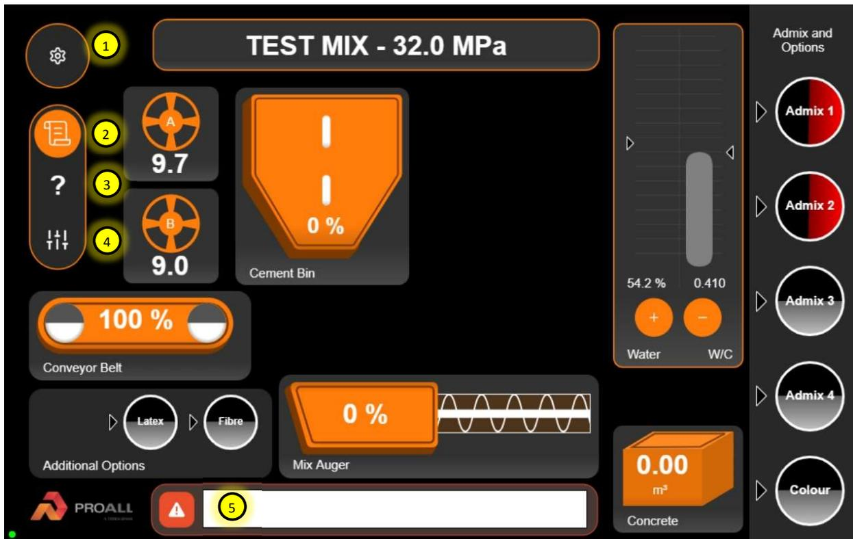
The Commander 2 display is touch screen only. There are no soft keys or buttons. Most mixer operation functions can be performed using the external keypads in the display box.
