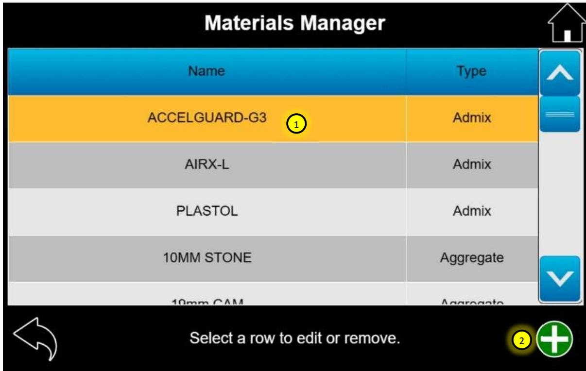
1. Materials manager is the first step in setting up the mixer for calibration and mix design entry. If no materials are entered into the table, then calibrations and mix designs can not be created.
