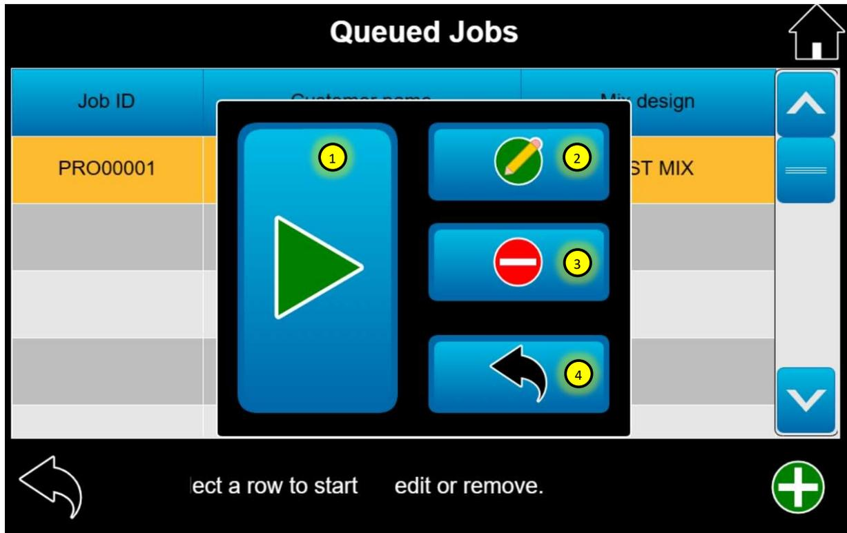
1. Start job (play) button. When this button is pressed the job details and mix design information will be loaded and the HOME page will display the mix design and subsequent component target settings will be calculated.
