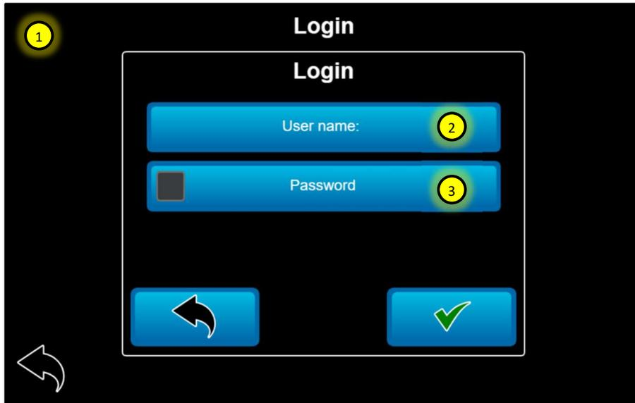
1. On first run when the Mixer Manager button is pressed on the HOME screen this login screen will appear.
