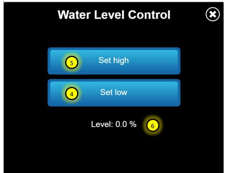
Note: Low water level alarm message is triggered when water is below 20%. The high water level alarm message is triggered when water is above 90%.
