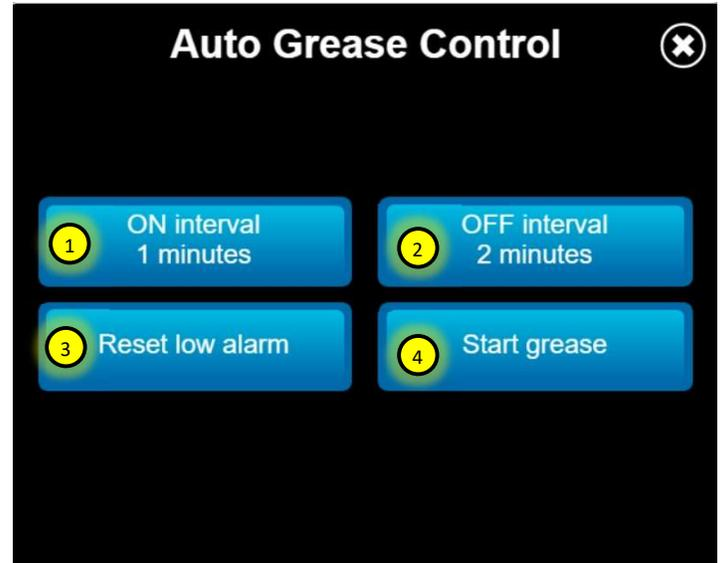
5. Manually start the chain oiler. In auto mode the chain oiler only cycles when the motor revolutions are surpassed.
