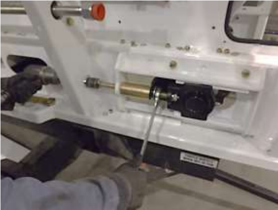
Figure 58. Adjust spring nut.
