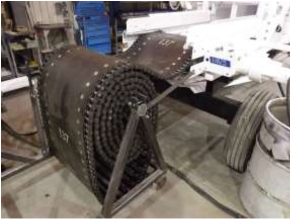
Figure 39. Example spindle used while unwinding the belt.
