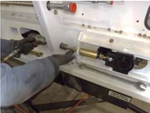
Figure 57. Adjust releasing nut towards threaded rod drive end.
