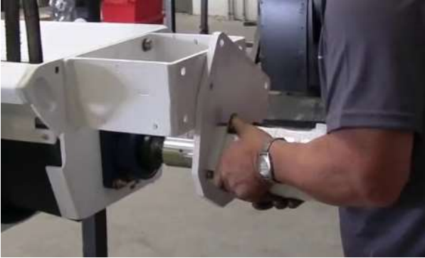
Figure 31. Install motor and motor mount plate
