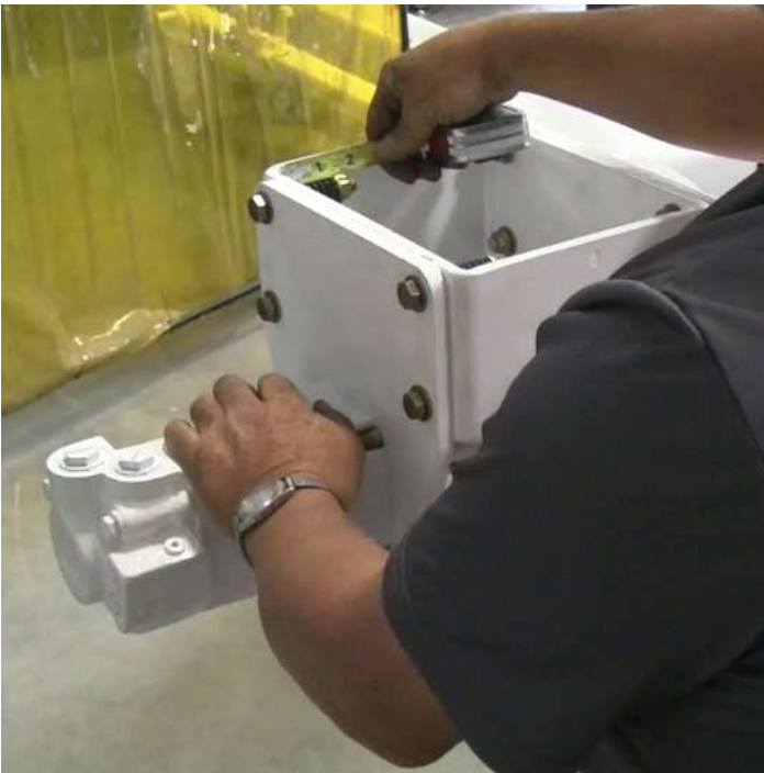
Figure 32. Compress springs to 1-3/8 inch
