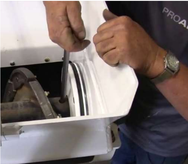
Figure 15. Use rod or drift to align holes in shaft and auger
