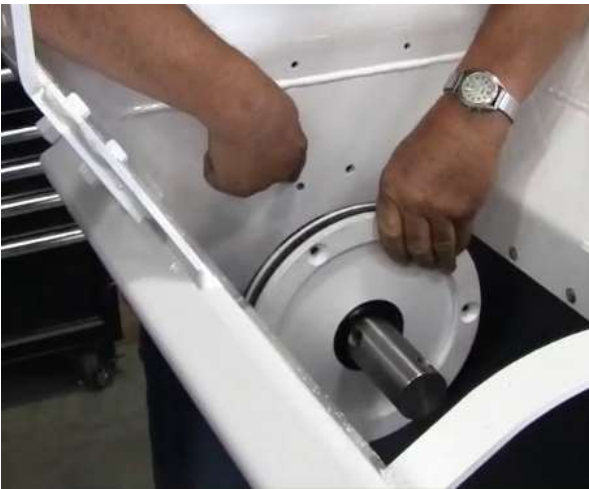
Figure 13. Align slot in seal assembly with grease hole in rear of mix auger frame
