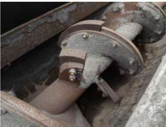
Figure 36. A newly replaced auger wear plate shown next to older wear plates. The older wear plates in this figure are not yet in need of replacement. New stir tab wear plates are shown on stir tabs that have worn down as far as possible without having to replace the stir tabs.
