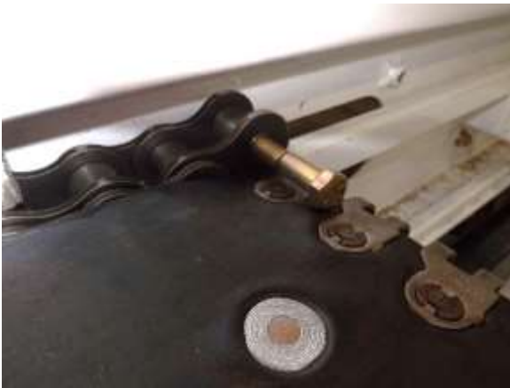
Figure 38. Add temporary bolts to the free end of the chain links.
