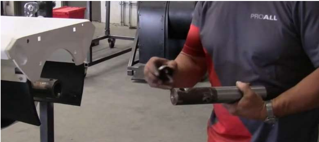
Figure 21. Place anti-seize on drive shaft
