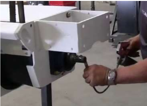
Figure 29. Place grease on drive shaft splines
