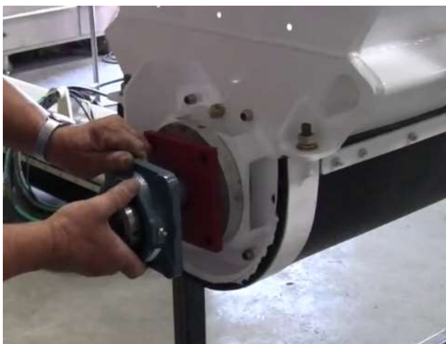
Figure 20. Install bearing with grease fitting to the right
