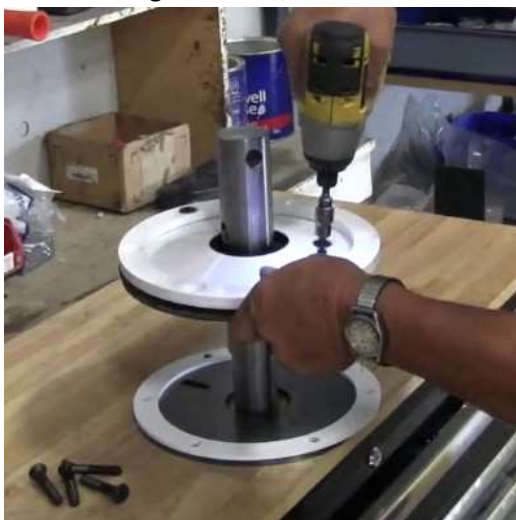
Figure 11. Use two bolts to align seal assembly
