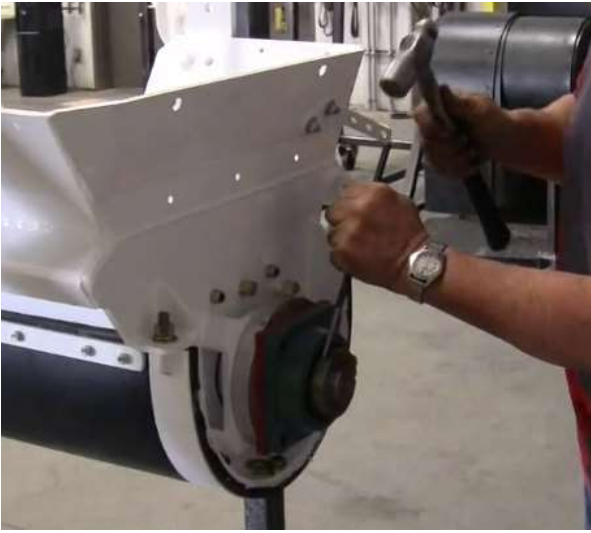
Figure 3. Loosen bearing collar
