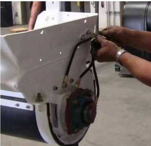
Figure 2. Remove grease hoses
