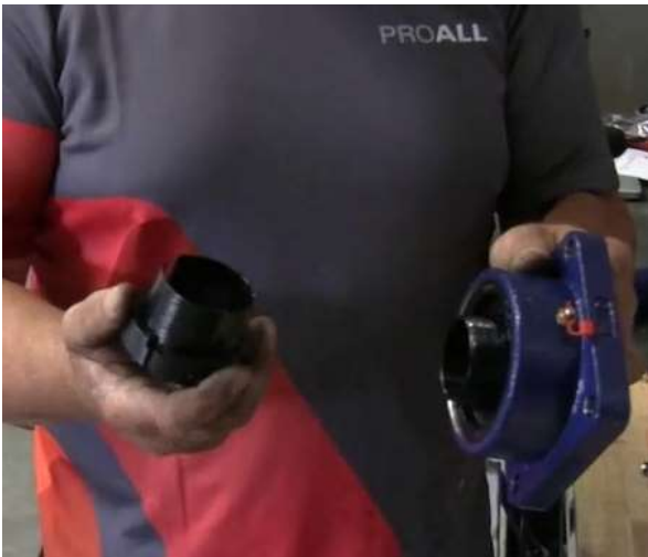
Figure 24. Remove bearing collar
