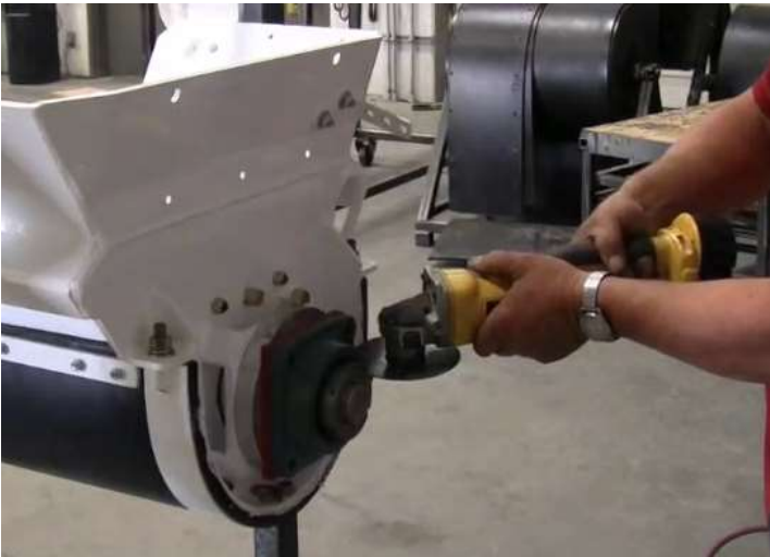
Figure 4. A cutting tool may be necessary to remove bearing
