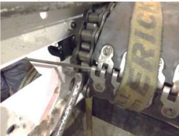
Figure 50. Tighten ratchet strap and bring upper and lower lacing teeth together along with lacing bar.
