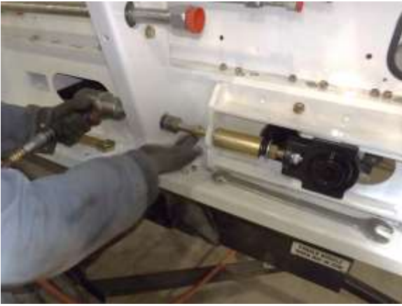
Figure 55. Adjust releasing nut.
