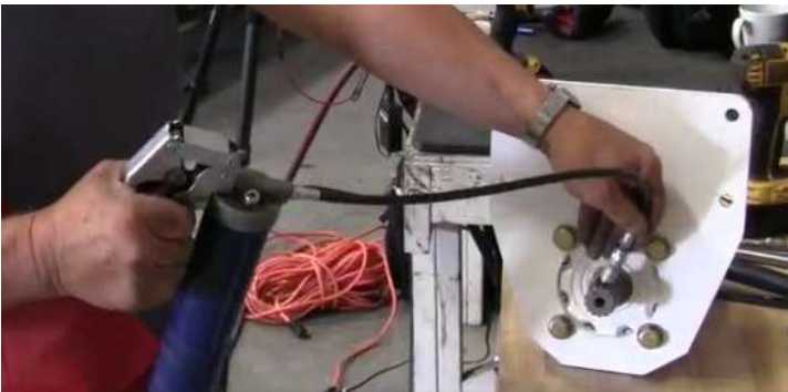
Figure 30. Place grease on motor splines
