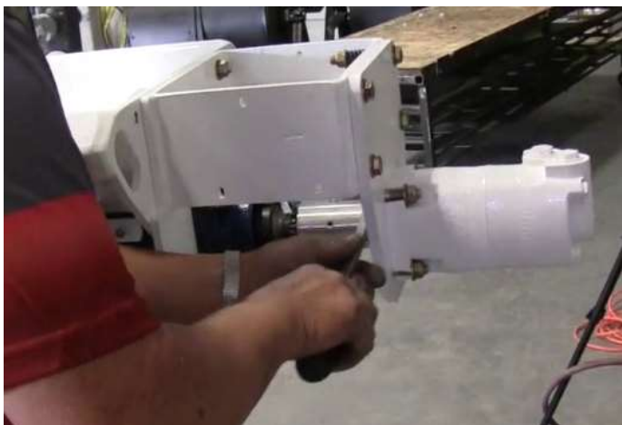
Figure 33. Move coupling with pry bar to test alignment of auger and bearing
