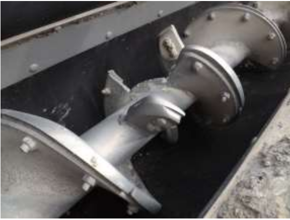
Figure 35. Typical worn stir tabs shown next to auger wear plates. The closest stir tab shown in this figure should have its wear plate replaced because the tab itself is worn as much as it can be. The furthest stir tab in this figure may be worn more as the stir tab wear is over 1/8 inch from the nut holding the stir tab wear plate to the stir tab.
