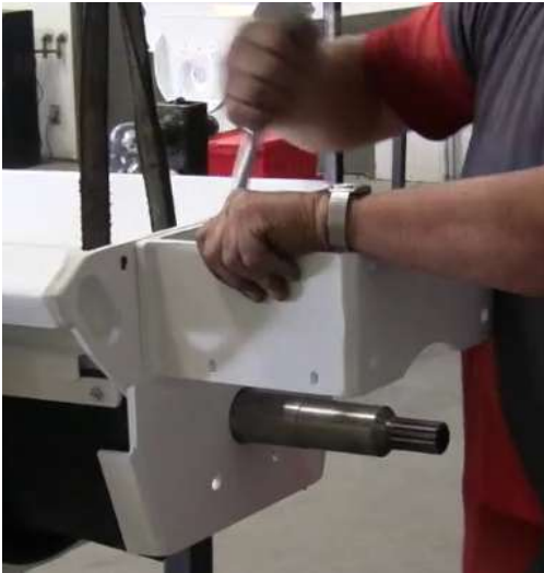
Figure 23. Install offset bracket
