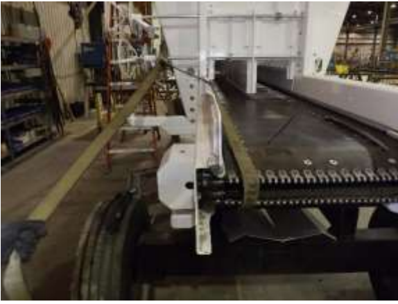
Figure 48. Installing ratchet strap for tightening belt lacing.
