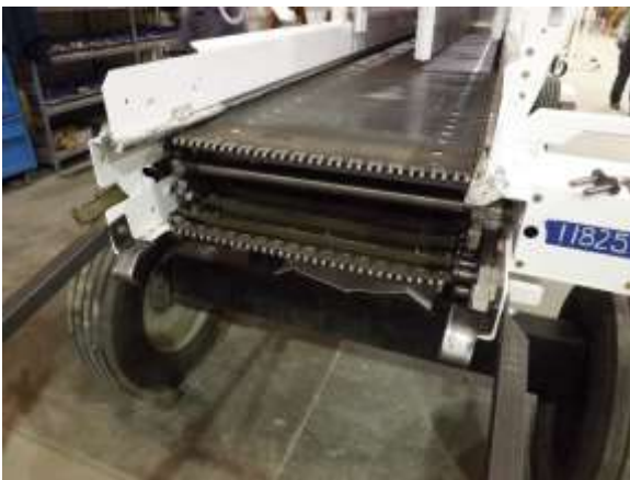
Figure 43. Belt lacing ends.
