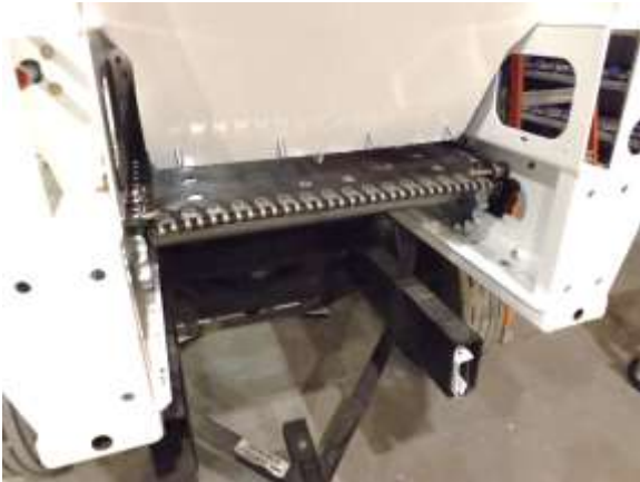
Figure 41. Remove bolts holding the chain links at this stage of the procedure.
