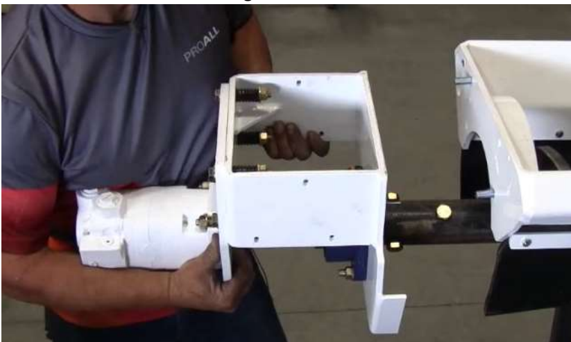
Figure 7. Separate mix auger from bottom of mix auger frame
