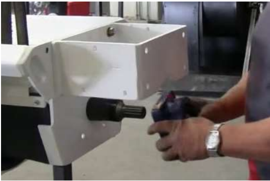
Figure 27. Installing bearing with grease nipple facing upwards
