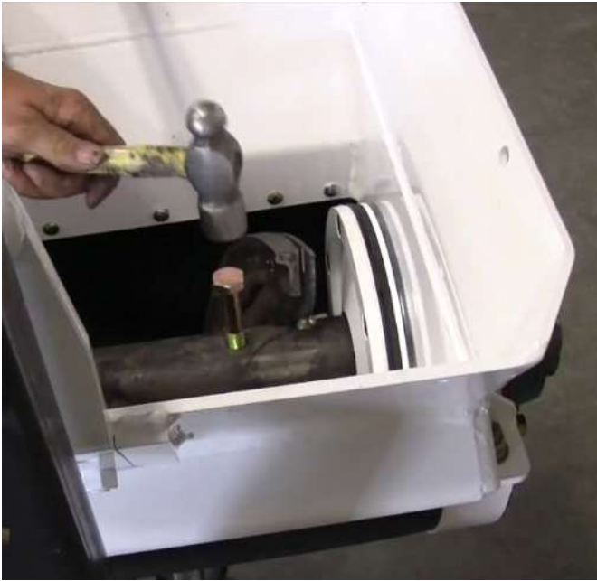
Figure 16. Tap bolts into place
