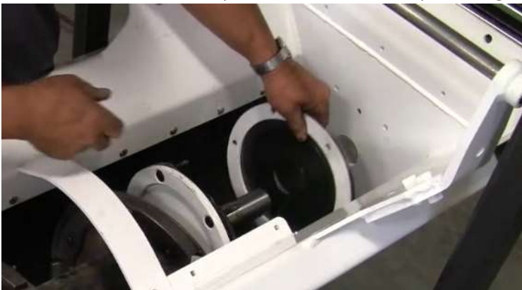
Figure 9. Remove wear plate and spacer ring
