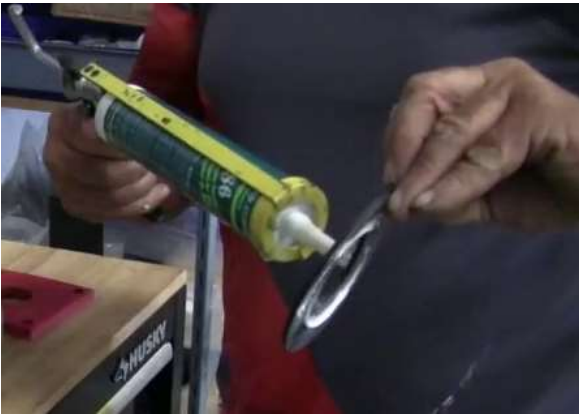
Figure 18. Place silicone on both sides of auger seal
