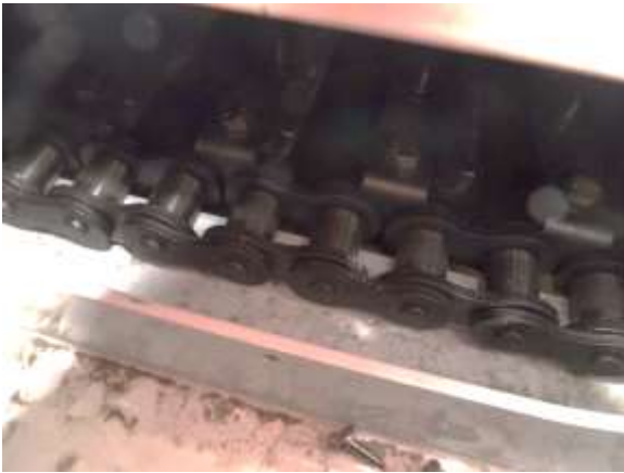
Figure 46. Chain properly resting on lower chain guide.
