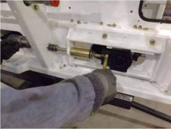
Figure 53. Loosen bearing nut.
