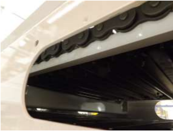
Figure 45. Chain properly resting on upper chain guide.
