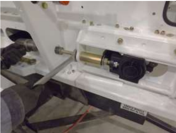
Figure 56. Loosen chain tensioner.
