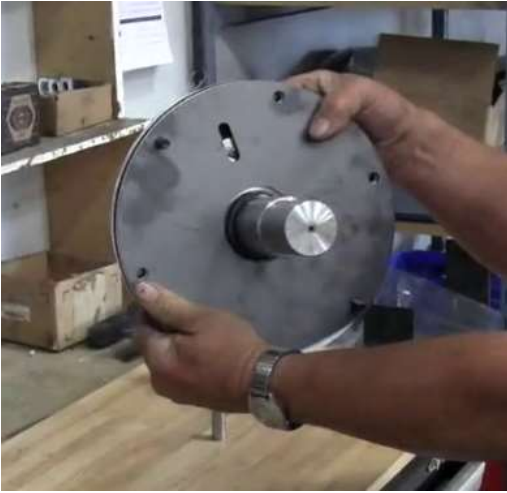
Figure 12. Slotted hole in wear plate towards the upper side of the mix auger
