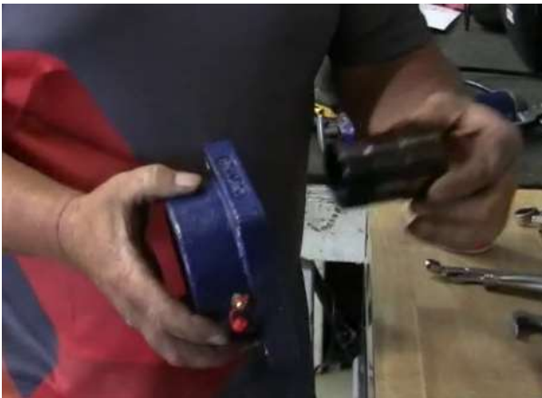
Figure 25. Remove bearing insert
