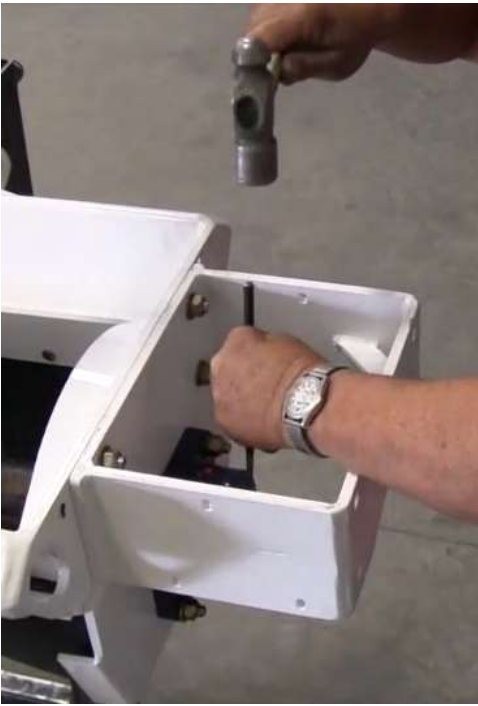
Figure 28. Tighten bearing collar
