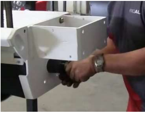
Figure 26. Place insert over drive shaft
