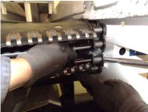
Figure 47. Install coupling links next to belt lacing.
