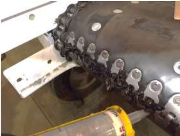
Figure 52. Caulk the lacing seam well into the lacing teeth.
