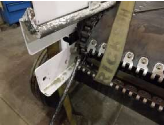
Figure 49. Pry bottom links towards rear of the mixer.
