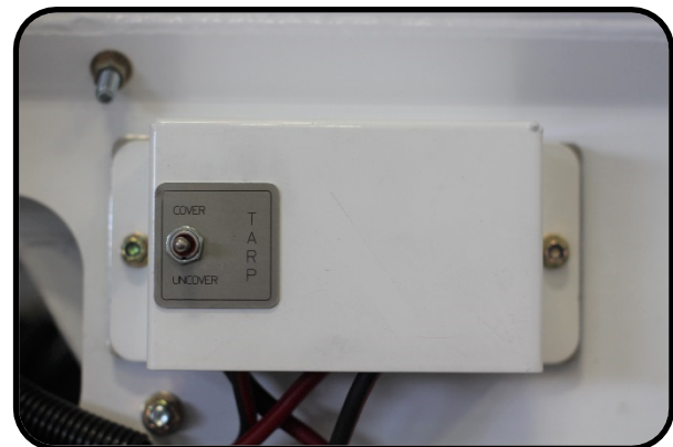
Figure 26. Tarp control switch.
