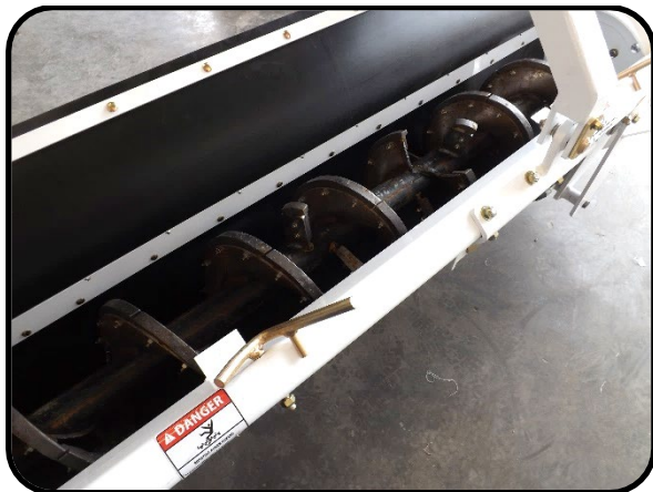
Figure 9. Auger cover open for cleaning.
