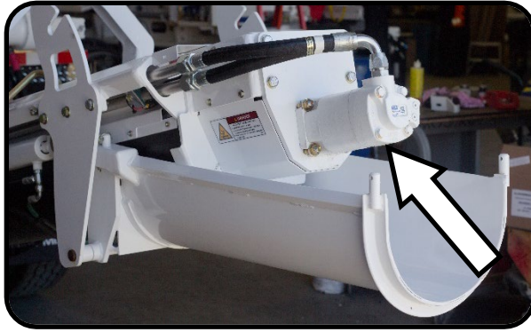
Figure 16. Mix auger top drive.
