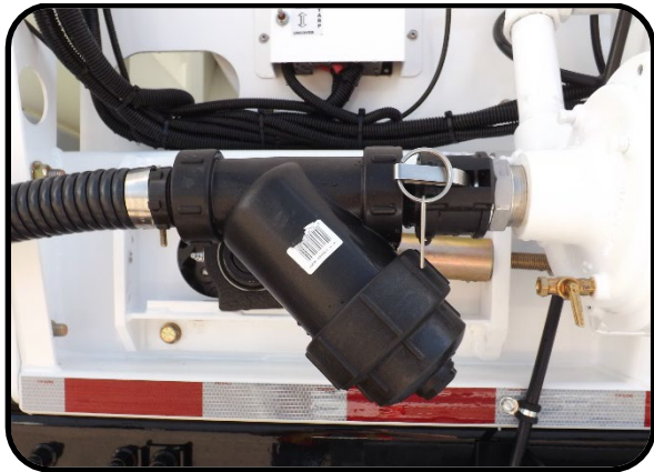
Maintenance 17. Clean water Y strainer.
