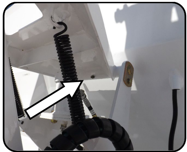
Maintenance 10. Lock arm grease.
