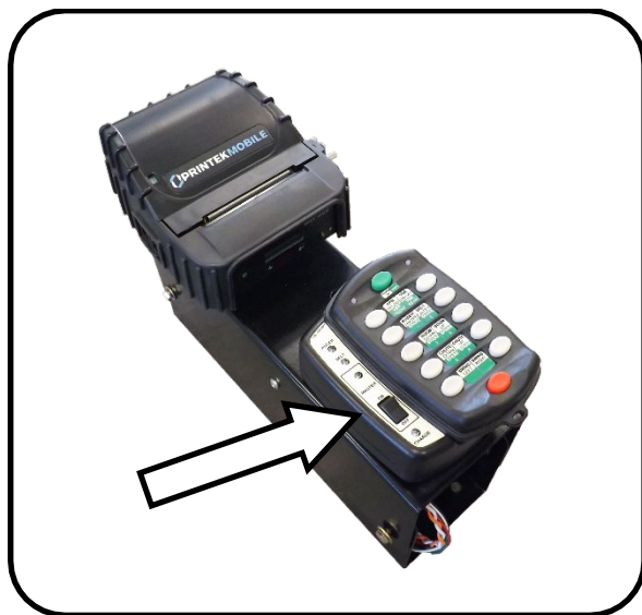
Figure 20. Remote receiver / printer stand master electrical switch
