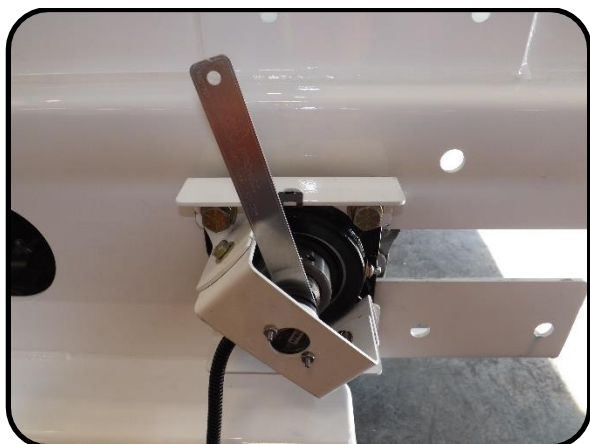
Figure 29. Speed sensor gap on conveyor drive shaft shown using a gap tool.
