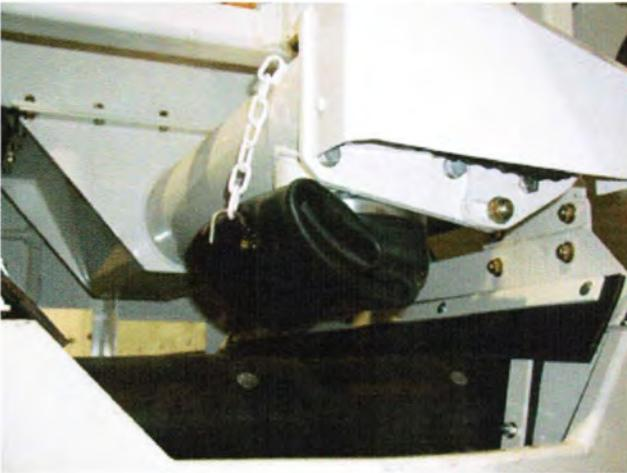
**Roll up cement drop tube as shown during wash out.**
