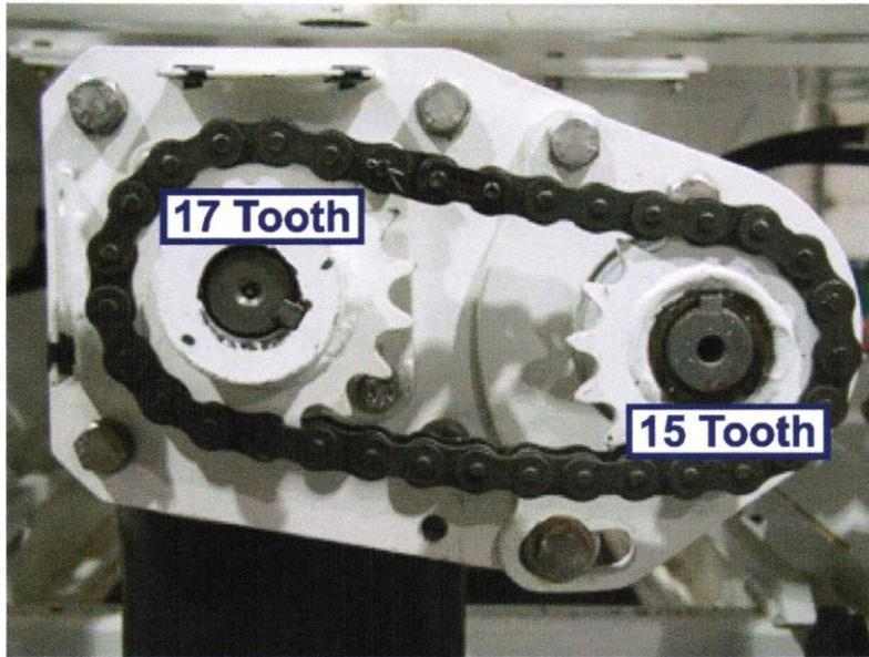
Cement sprocketing shown above, can be interchanged by the operator to increase cement delivery.
