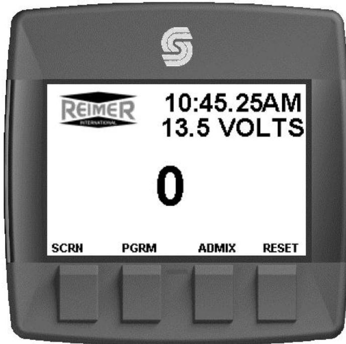
SCRN – Switch to Run Screen, PGRM - Switch to Program Screen
