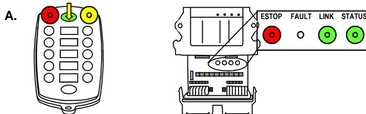
Once the ID Code has been downloaded, the RED (Battery) light and the YELLOW (Active) light on the transmitter will go out. The (Link) light on the receiver will change from GREEN to RED.
