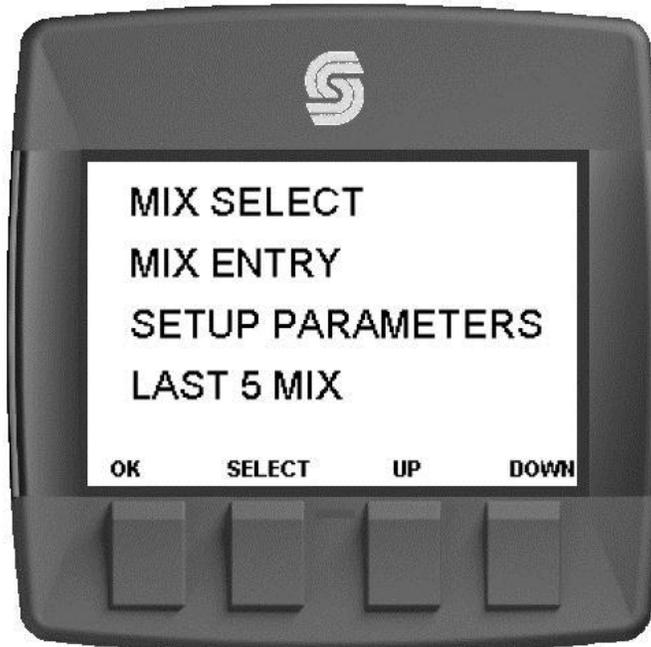
OK – Switch to Run Screen, SELECT – Switch to highlighted screen,
