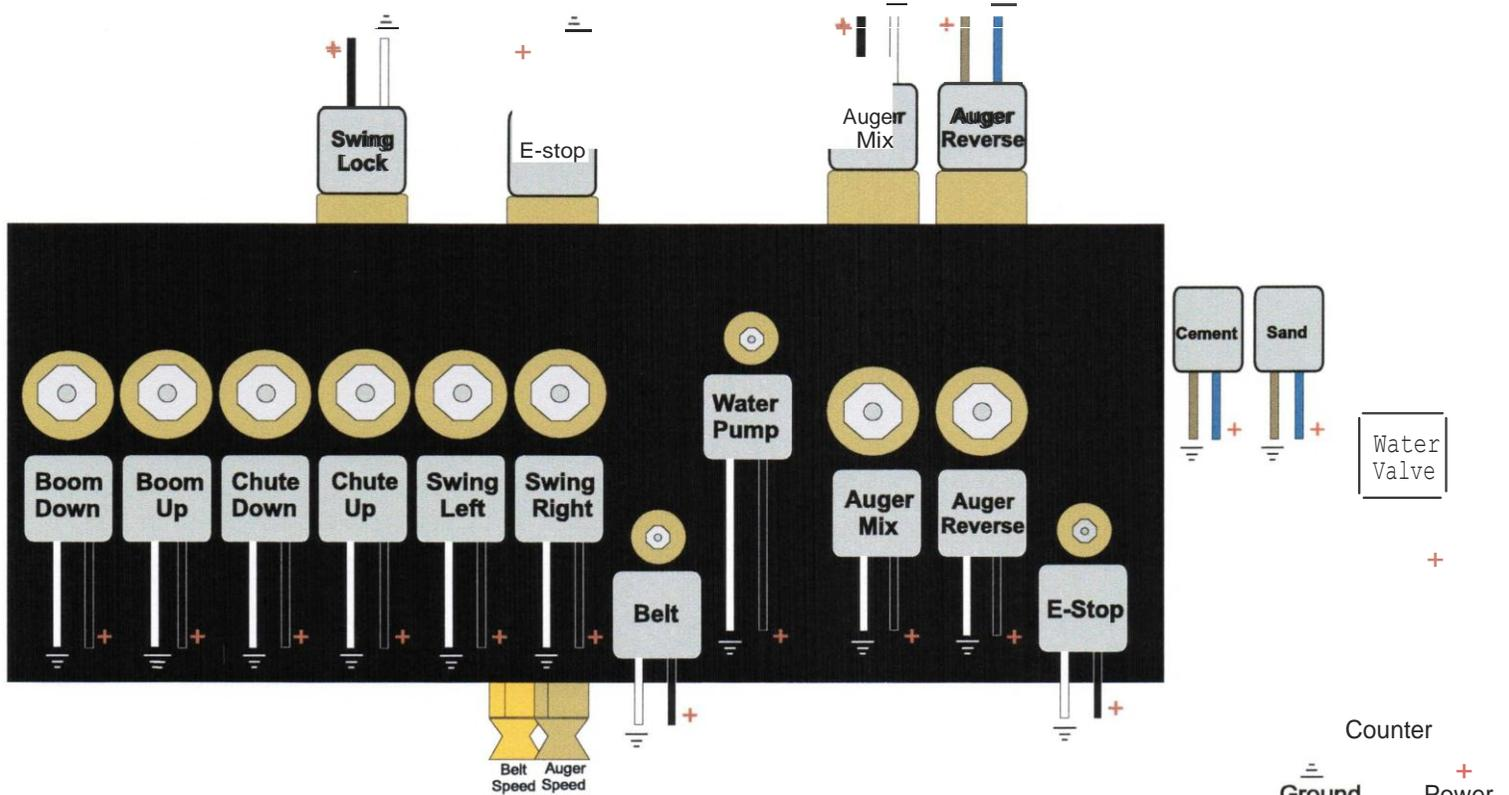
Each solenoid connector has 2 wires
