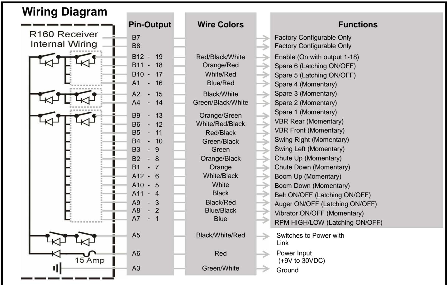
**Outputs:** 19 solid state, high-side driver outputs, 5A max. per pin and 7A max per bank, total combined current 15A
