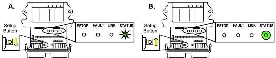
**NOTE:** If left idle in Setup Mode for over 30 seconds, the receiver will time out. The (Link) light and (Status) light will flash RED rapidly. To return to Setup Mode, repeat step 4.
