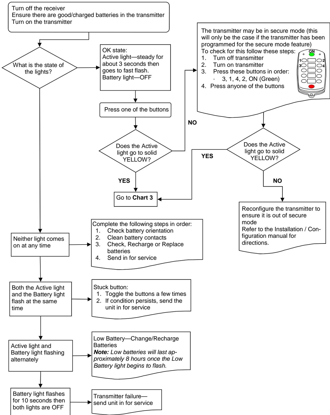
Testing the Transmitter / Receiver Communication
