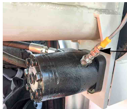
MOTOR OUTPUT cable connection on proportional control valve
